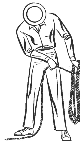
FIG. 110. Coiling a rope, second position.
