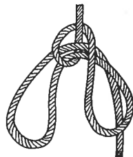
FIG. 108. Bell-ringer's knot. For temporarily tying up the lower end of a hanging rope.
