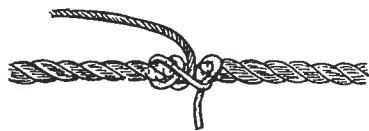
FIG. 49. Rolling hitch.* For fastening a rope to another rope or a pole parallel to it. For attaching a life-belt rope to a hanging life line. Grips tightly if pulled in direction shown, but is easily moved along rope or pole when strain is relieved.
