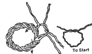
FIG. 62. Grommet. An endless rope of one strand only, it makes three complete loops. To terminate, divide strands as shown and tuck as in short splice.
