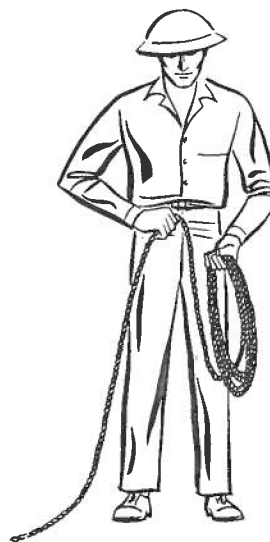
FIG. 109. Coiling a rope, first position.
