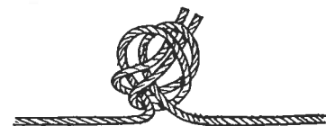
FIG. 15. Overhand knot, or rosette knot. For joining two ropes. Will not slip but is of low efficiency.
